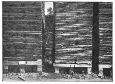
Frg. 89.—Lumber piled so as to form "chimney" or flue near center of stack from bottom to top.
